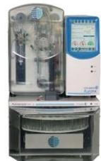
Move over Total Kjeldahl Nitrogen (TKN) testing. There's a new total nitrogen analyzer in town, and it draws a quick analysis time of 10-15 minutes...
