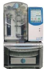
The Aurora 1030W TOC Analyzer uses the proven heated persulfate wet oxidation technique to analyze organic contamination levels in liquid samples. The instrument can be programmed and calibrated to analyze samples containing organic carbon at levels as low as 10 ppb and as high as 30,000 ppm. In addition to its wide range, the Aurora 1030W has an extremely high daily throughput. Up to 300 samples can be analyzed in a 24-hour period (dependent on method and application).
